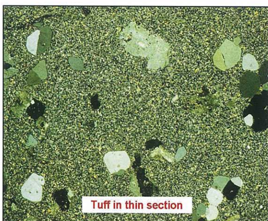
Figure 12 Crystal ash tuff in thin section
