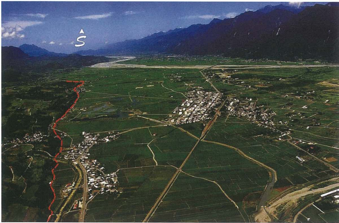
Figure 8. An aerial view looking southward along the Longitudinal Valley above the Chihshang Town. The Central Range is located to the right-hand-side and the Coastal Range is located to the left-hand-side of the Longitudinal Valley, respectively. The surface traces of the Chihshang fault trending N-S generally follow geomorphic scarps and boundary between the rugged hills of the Coastal Range and the flat alluvial deposits of the Longitudinal Valley.
